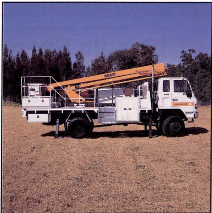
12m Truck Mounted Elevating Work Platform
