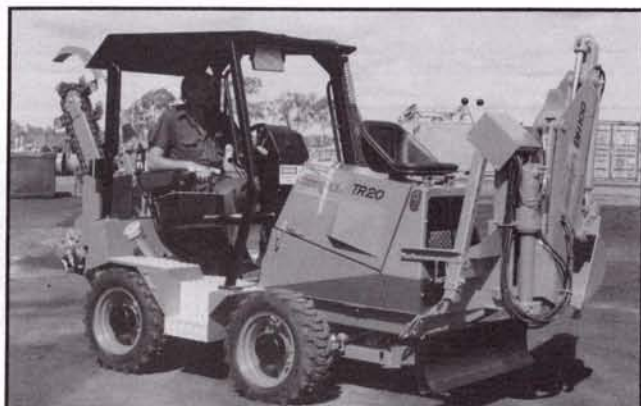
The new Austoft Mustang TR20 trenching machine, powered by a 22kW diesel engine.
