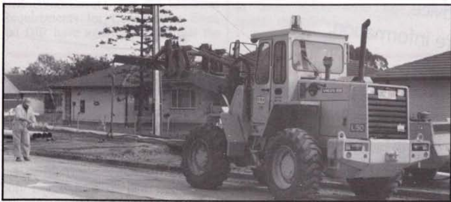
Volvo BM L50 front end loader fitted with material handling arm for pipe laying application. The unit is powered by a 82hp Volvo D45B Volvo diesel engine.
